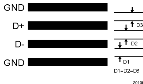
FIGURE 10. Ideal Diode Trace Layout
